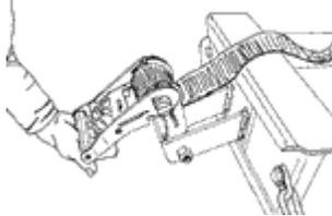
3. Lift ratchet handle to full extended position and unroll straps from ratchet. Return ratchet handle to the down position.
