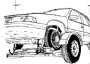
11. Hook up safety chains from tow dolly platform to the frame of towed vehicle directly above the area where chains are mounted on tow dolly. Allow slight slack in the chains to provide for suspension movement on the towed vehicle.
