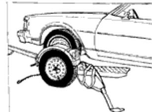
4. Remove wheel straps and safety chains from towed vehicle.
